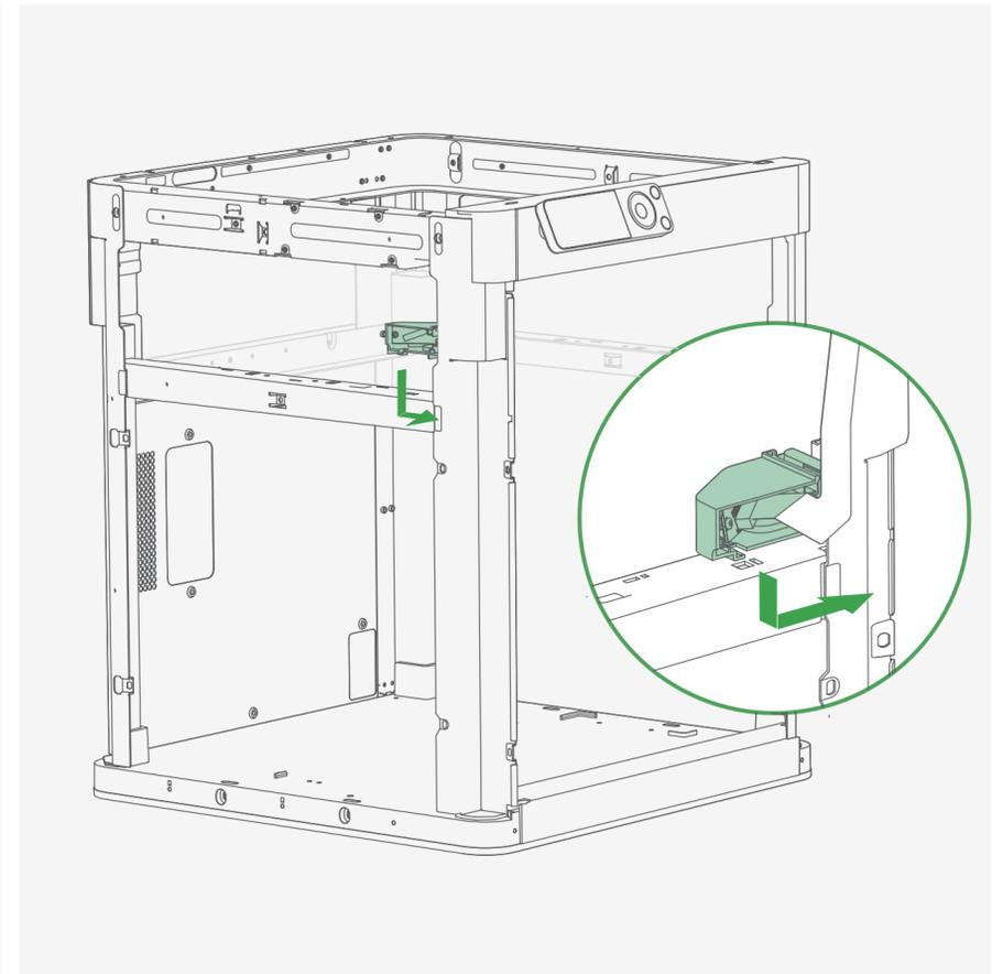
Plug the camera into the port as pictured, then lock it by pushing it to the right.
