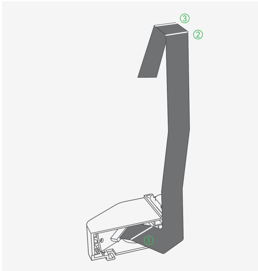
Bend the FPC cable three times along the white lines as shown above.
