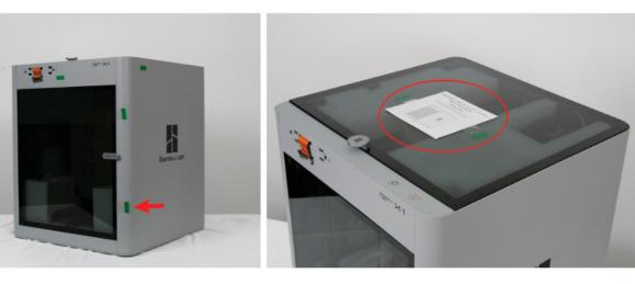
3. Carefully remove the glass cover plate and the protective foam inside the printer, and then take out the accessories box.
