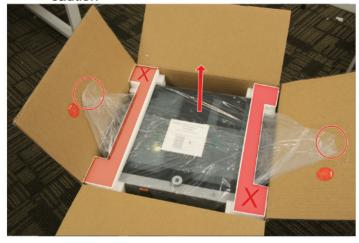
Remove the plastic bag and peel off all the green stickers surrounding the printer. At this point, it is recommended to review the quick start before continuing.
