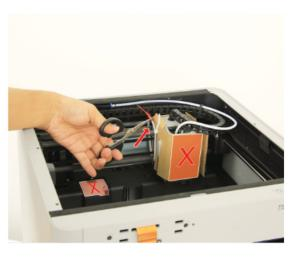
Open the front glass door, remove the two protective foam pieces and the desiccant bag and take out the PC sheets. Remove the note attached to the sheet that reminds you to use a glue stick on the sheets.
