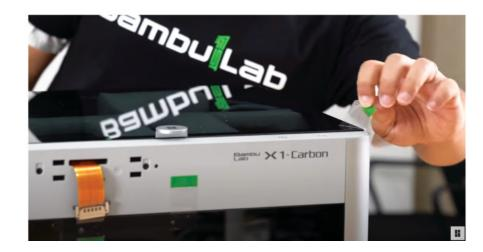
Remove the top glass cover to reach the protection foam holding the AMS attachment safe during shipping.
