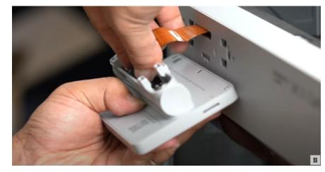
Connect the PTFE tubes and the cables to the machine. Then you can start the printer and begin the initial automated calibration process.
